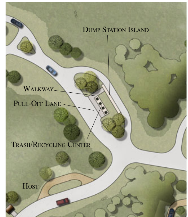
A common dump station design includes a dumping station on one end and a fresh water fill on the other, as this MN DNR design illustrates.
